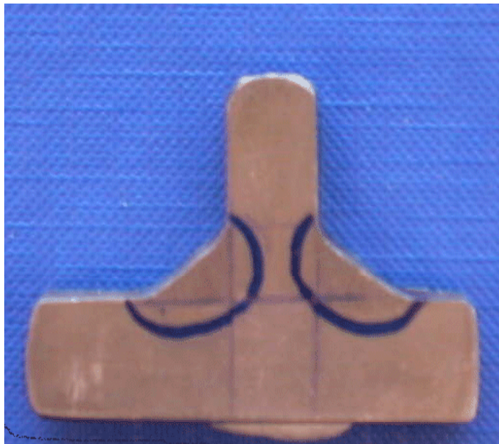
T-junction section, highlighting HAZ region
