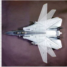
High-lift, variable sweep wing
