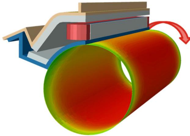
**Figure 2:** Temperature contour of induction heated fuser
