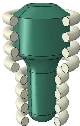
**Figure 1:** Work coil and work piece for metal hardening example
