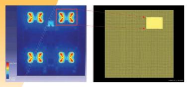
Using ML to automate the detection of chip hot spots by applying fine meshes where they are needed.
