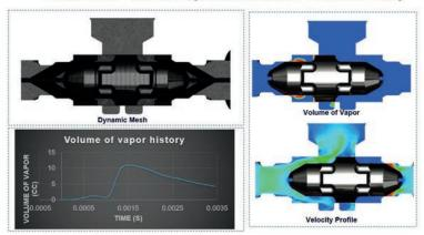
Subsea valve cavitation study
