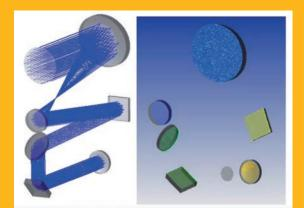
Using the Ansys Zemax OpticStudio STAR software to add deformations (generated by finite element analysis) to the optical model of a mirror system
