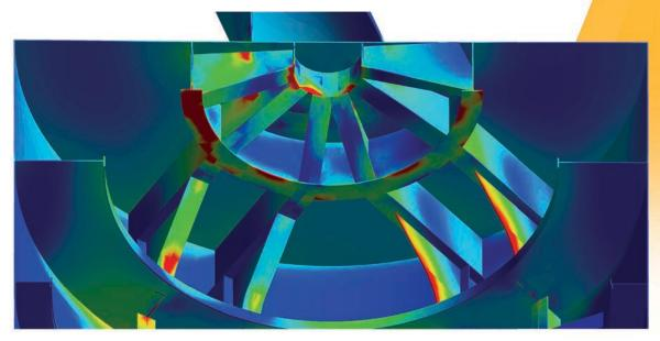
Interior view of the starboard column, showing the internal reinforcements under the main mast connection
