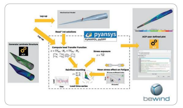
Figure 1. Illustration of Bewind's integration of PyAnsys with two templated load cases to compute load transfer functions at varying stress levels at each composite layer using the binary result files of a rotor blade model.
