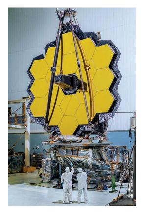
The primary mirror of NASA's James Webb Space Telescope, consisting of 18 hexagonal mirrors, looks like a giant puzzle piece standing in the massive cleanroom of NASA's Goddard Space Flight Center in Greenbelt, Maryland.
