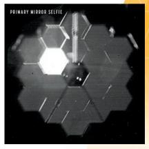
"Selfie" taken by JWST of its primary mirror, captured by a special lens within its near-infrared camera (NIRCam)
