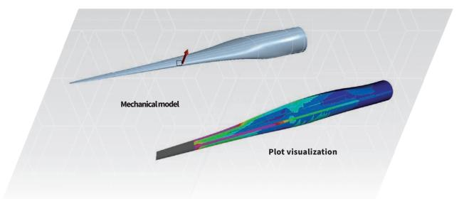
When materials experience fatigue, small cracks initiate and grow under the influence of cyclic loading. Even though the applied load is less than the tensile strength of the material, the repeated, cyclic nature of the loading can cause fracture and failure. Fatigue loads come in two categories: constant and variable amplitude. In real-world scenarios, variable amplitude cyclic loading is more common.
