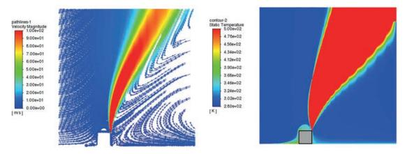
Figure 4: Velocity colored streamlines and temperature contours for a 2D planar thermal pressure release device (TPRD) model with 5 m/s wind coming from the left
