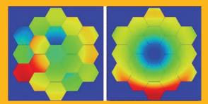
An optical model of JWST-like primary mirror segments, with piston errors (left) and in its perfectly aligned state (right)
