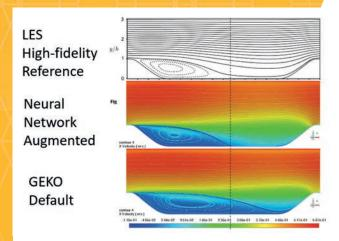
Turbulence modeling using large-eddy simulations and Reynolds-average Navier-Stokes (RANS) equations, with generalized k-omega (GEKO) models.
