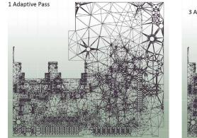
Figure 7a. Meshes due to adaptive refinement after Pass 1 in Slwave
