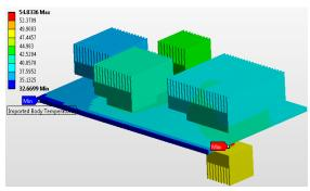
Figure 20. Icepak temperatures mapped onto the board in Mechanical
