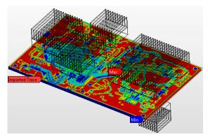
Figure 19. Imported layer metal with heat sinks
