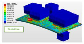
Figure 23. Elastic strain
