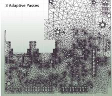
Figure 7b. Adaptive mesh after three passes
