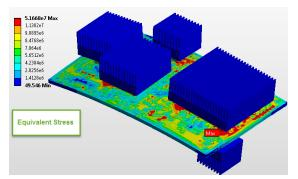
Figure 22. Thermal-induced stress
