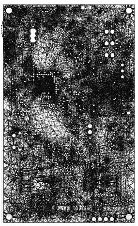
Figure 9. Final mesh of the PCB
