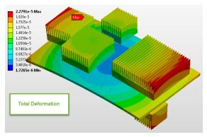
Figure 21. Thermal-induced deformation in Mechanical
