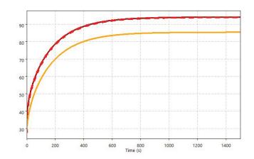
Figure 13: Result showing component warmup of the U half-bridge simulated thermal transient curve
