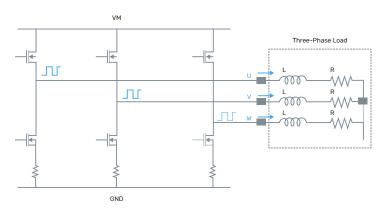
Figure 14. Three-phase load connected to the inverter
