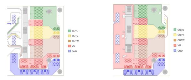
Figure 5: EVALSTDRIVE101 second inner-layer PCB
