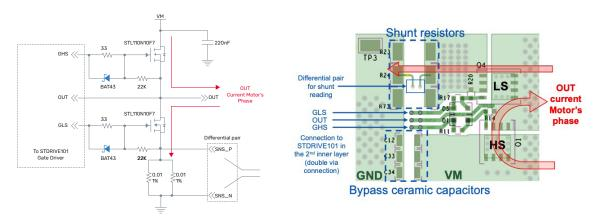
Figure 7: Schematic of one-half bridge in the EVALSTDRIVE101 and associated layout pattern
