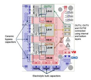
Figure 3: EVALSTDRIVE101 top-layer PCB
