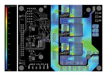
Figure 11: Current density resulting from DC current loops
