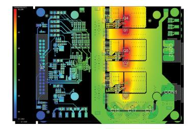
Figure 12: Result showing steady-state PCB simulated top layer temperature map
