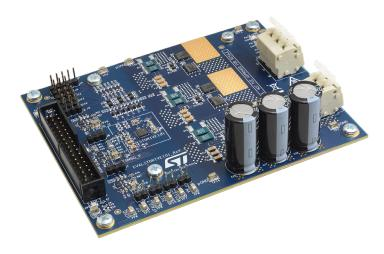
Figure 1: EVALSTDRIVE101 demonstration board
