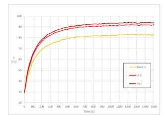
Figure 17: Measured thermal transient curve - EVALSTDRIVE101 warmup at 15A<sub>rms</sub>
