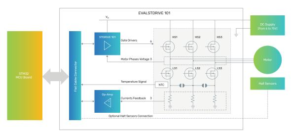
Figure 2: EVALSTDRIVE101 basic block diagram
