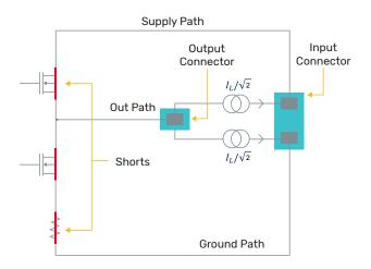
Figure 9: PCB current loop modeling
