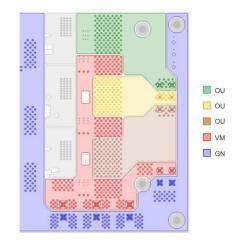
Figure 4: EVALSTDRIVE101 first inner-layer PCB
