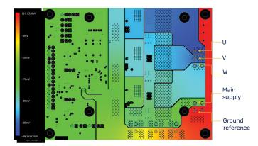
Figure 10: Voltage drops resulting from DC current loops
