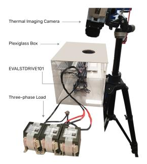
Figure 15: Setup for the thermal characterization of the board
