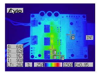
Figure 18: Thermal measurement - EVALSTDRIVE101 steady-state thermal image
