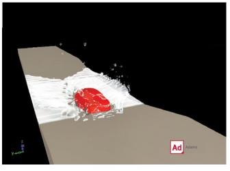
Figure 10. Adams – scSTREAM prediction of a dynamic vehicle suspension movement through a puddle
