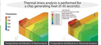
Temperature distribution from scSTREAM is mapped on to the mesh of structural analysis. The stress on solder connection is calculated using structural analysis.
