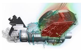
Hexagon Leica RS 6 Scanner. Internal thermal convection & conduction
