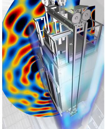
Bust as we didn't just want to identify the issue, but also try out design improvements, we created a 180-meter long CFD simulation model containing two shafts and coarse models of our elevator cars. This provided a complete, detailed, view of the flow model, and the sort of turbulence we could expect in and around the shafts of our "giant whistle".
