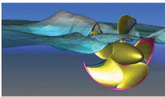
Figure 12. MSC Nastran - scFLOW prediction of propeller with free surface and cavitation
