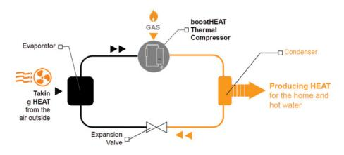
Figure 1. The BoostHEAT heat pump boiler principle
