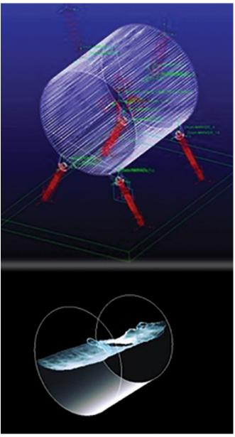
Figure 9. Adams - scFLOW prediction of dynamic sloshing of liquid in a tank
