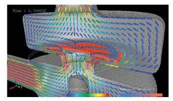
Figure 11. FSI analysis using Marc and scFLOW of a Valve with an Elastic Membrane deformed by flow
