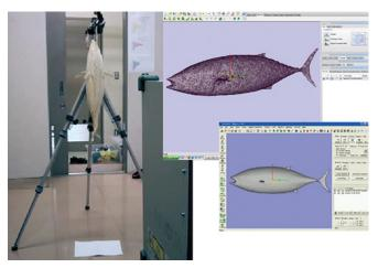
Figure 1. Tuna being scanned on a 3D scanner in Prof Takagi's laboratory with resultant geometry and surface mesh representation
