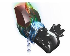
Hexagon Leica RS 6 Scanner. Thermal convection around the cooling grill
