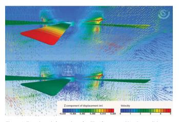
Figure 2. Transient deformation of ceiling fan caused by air-conditioner wind evaluations
