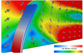
Figure 4. MSC's Nastran – scFLOW - Marc Co-Simulation of a flap bending and twisting in a crossflow
