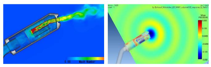
Figure 6. MSC's Cradle CFD and Actran Acoustics co-simulation for an Automotive Exhaust and Muffler Aeroacoustics Prediction
