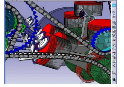
Coupled simulation with functional model for chain tensioner / actuator
