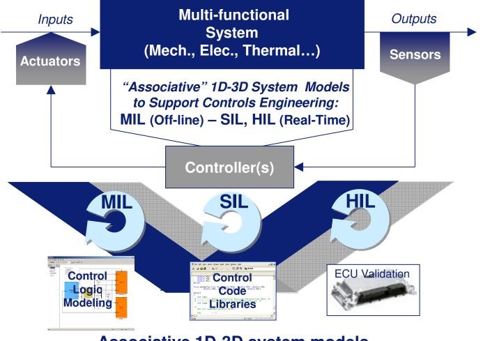
Associative 1D-3D system models to interconnect mechanical and electronics/control engineering
