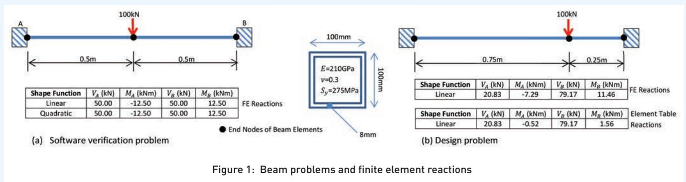
Figure 1: Beam problems and finite element reactions
