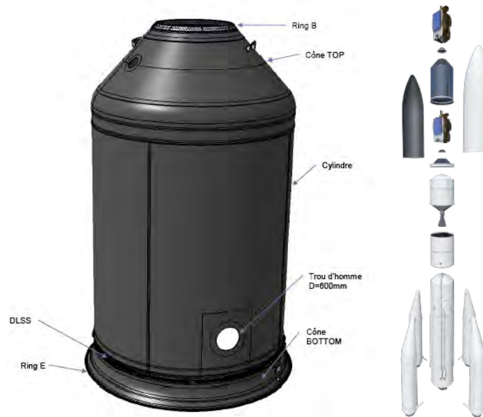
Figure 1: Ariane 6's Dual Launch Structure (left) and location within the launcher (right)
