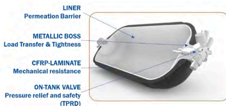
Fig2: Type IV high pressure vessel design
