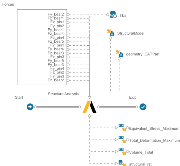
Figure 5: Workflow for structural analysis. CAE model is referenced from SPDM using external data source connector.
