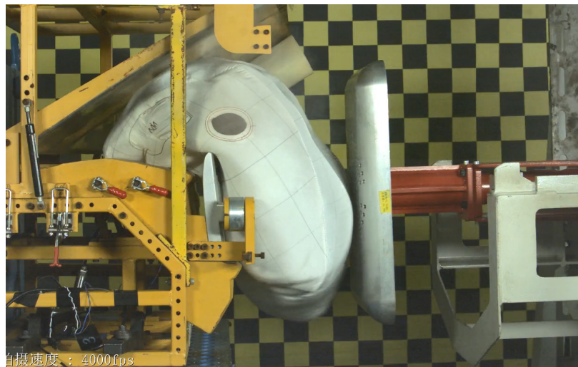
Figure 4: passenger airbag linear impactor experimental test (courtesy Yanfeng)
