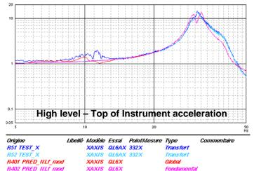
Overall shape matches well with test results despite two predicted peaks versus only one peak being measured. Axial excitation/response
