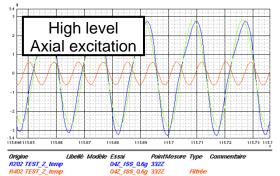
402 TEST\_Z\_temp 04Z\_ISS\_0.6g 332Z Filtrow Top of Instrument dummy acceleration on main SASSA mode at ~57Hz
