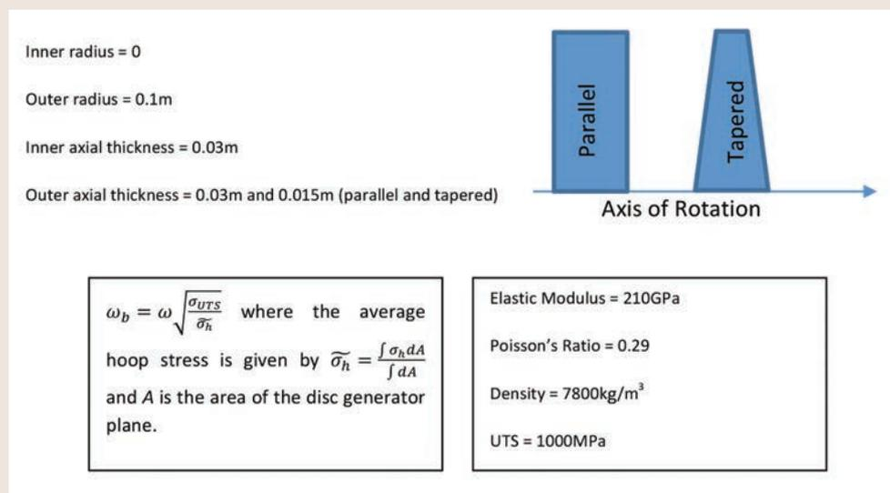
Figure 1: Generator planes for the axisymmetric finite element analysis of two rotating discs
