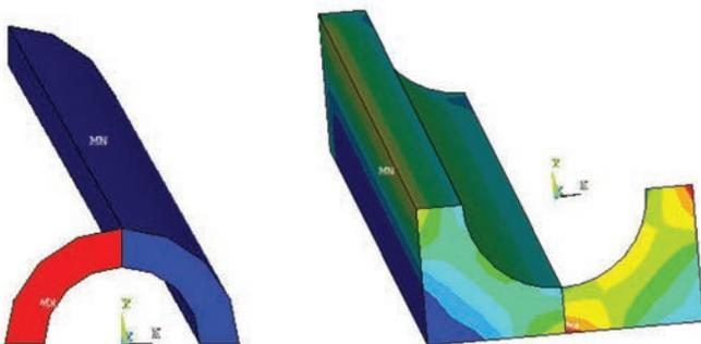
Figure 1:  $S_{zz}$  stresses for two cylinder geometries
