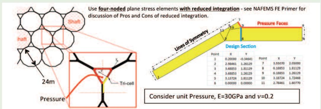
Figure 1: Shaft and tri-cell honeycomb and a basic finite element model
