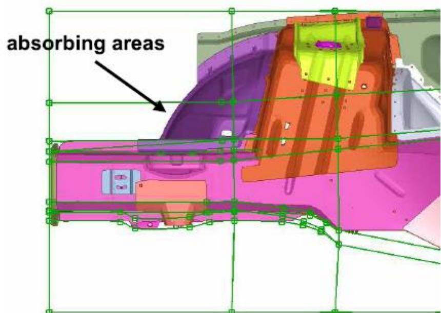
Figure 7: Rail modified shape
