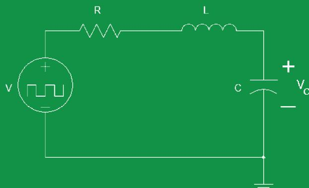
Figure 1: Equivalent R-L-C circuit model
