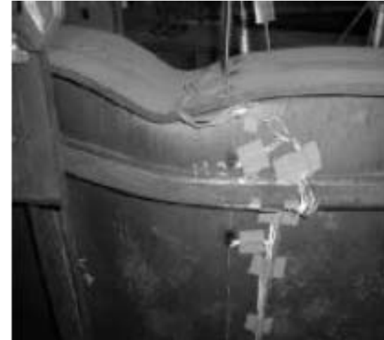
Lateral torsional buckling observed in the experiment
