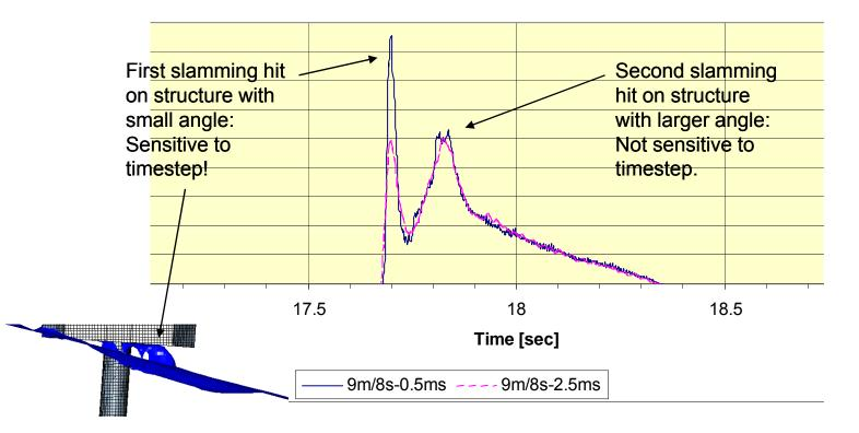
Example of slamming case very sensitive to timestep due to small slamming angle between water and structure
