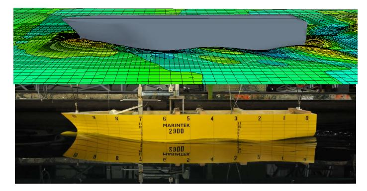
Comparison between CFD and model test of generated waves from a vessel
