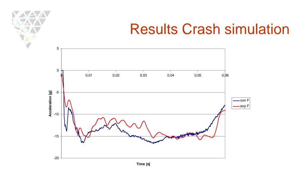
• The behaviour of the virtual B-Pillar is slightly stiffer compared to experiments
