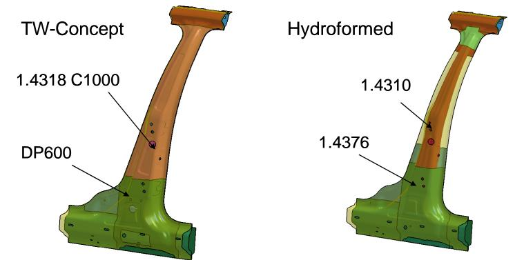
• Both concepts were simulated, produced and crash tested.
