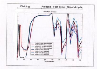
Figure 39 The evolution of von Mises stresses during simulation represented in four nodes. Two of them, 12178 and 12197, is located in the center of the weld, and the other two in the heat effected zone. The continous lines are for the welded simulation and the dashed lines are for the non-welded simulation
