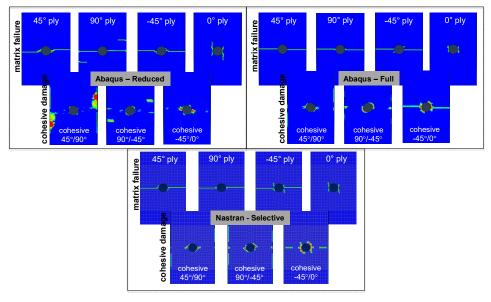
Figure 3. Comparison of the predicted intra-laminar and inter-laminar damage distribution at the critically damaged state (at max load) for the three different code combinations.
