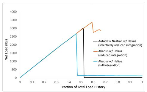
Figure 2. Comparison of the predicted response of the Open Hole Coupon using three different code combinations.
