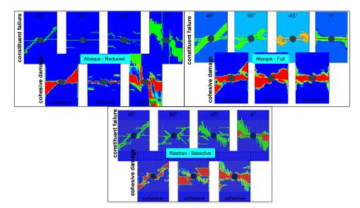
Figure 4. Comparison of the predicted intra-laminar and inter-laminar damage distribution immediately after the global failure cascade (large load drop) for the three different code combinations.
