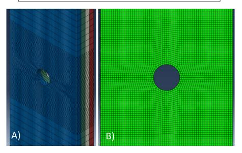
Figure 1. Finite element mesh of a laminated composite open-hole tension coupon. A) Oblique view showing the discrete layer mesh (one element layer per composite ply), B) close-up planform view of the refined mesh around the circular hole.
