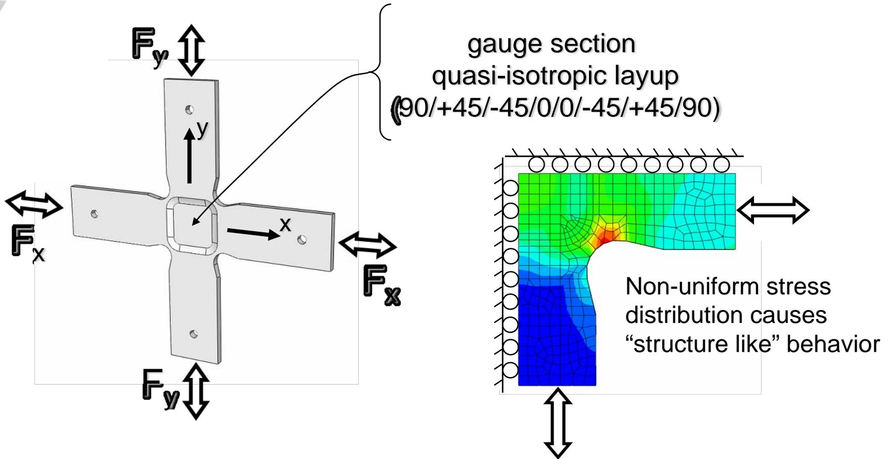
For various fixed ratios of  $F_x/F_y$ , incrementally increase the applied loads until structural failure occurs.
