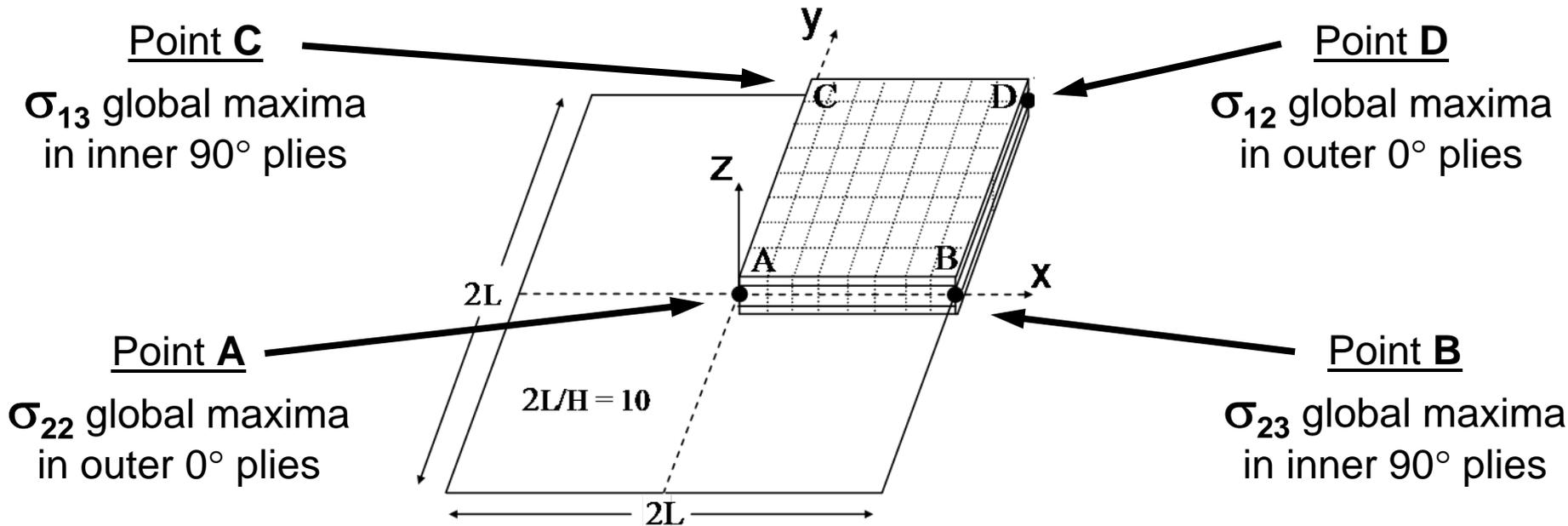
*The epicenter of damage evolution is dependent on the distribution of stress components and the relative strength of the composite material in the various modes of deformation*
