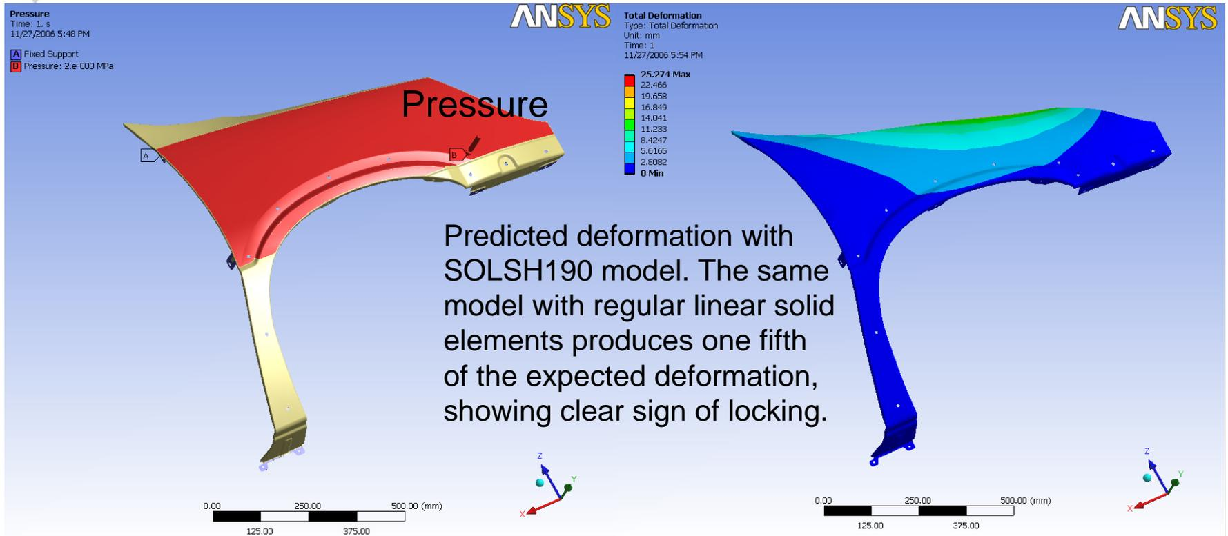
Mid-surface extraction based shell meshing may not be practical for parts with complex geometry and variable thicknesses, or when design parameters still need constant modification.
