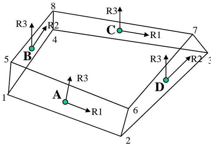
NTS strains at the centroids of four element faces:
