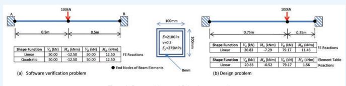
Figure 1: Beam problems and finite element reactions
