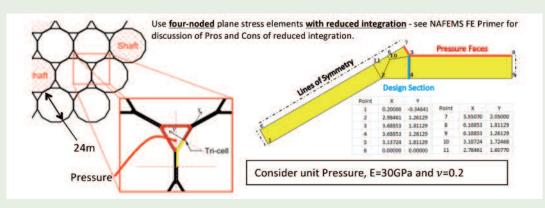
Figure 1: Shaft and tri-cell honeycomb and a basic finite element model
