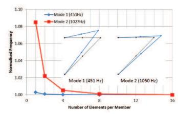
Figure 4: Convergence of frequency for truss structure modelled with constraint equations
