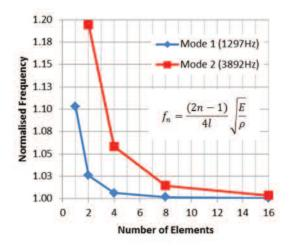
Figure 2: Finite element approximations of the first two modes for the test structure (CS1)
