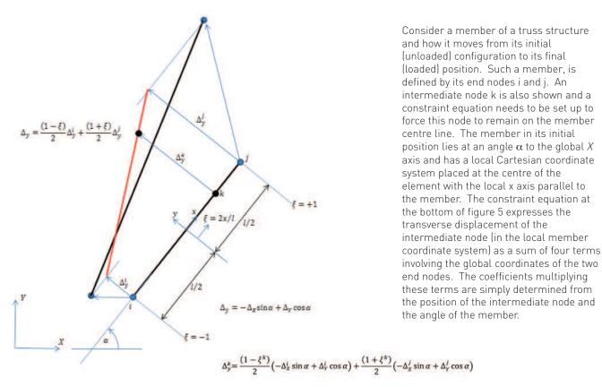
Figure 3: Constraint equation for an intermediate node
