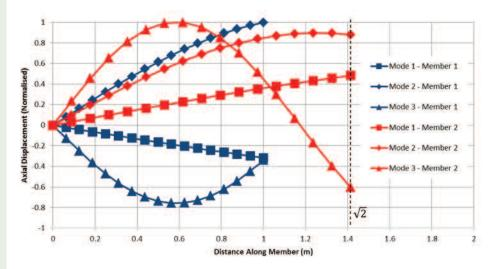
Figure 5: Member axial displacements for the 16 element per member mesh of the truss structure
