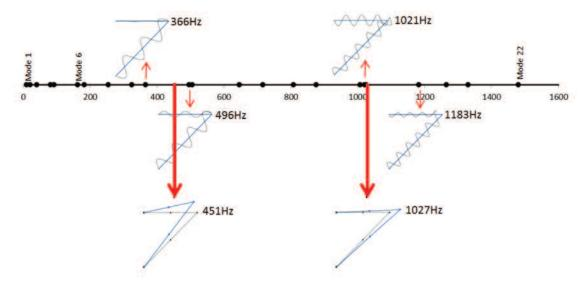
Figure 6: Frequencies and modes for truss structure modelled with beams and bars
