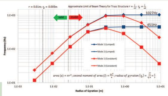
Figure 7: Frequency variation with radius of gyration for beam model of truss structure
